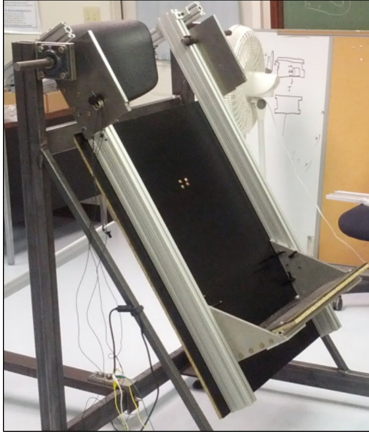
Figure B.3: Leg Platform. Foot platform can be adjusted to the height of the participant
