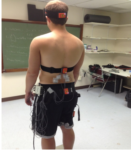
Figure 3.1: Electrode placement on participant's back
