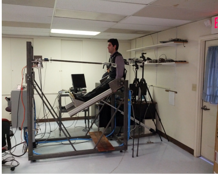
Figure 3.4: Participant's legs were raised to 70 percent of their maximum flexion angle of their trunk for stress relaxation portion of experiment and remained in that position for four minutes.
